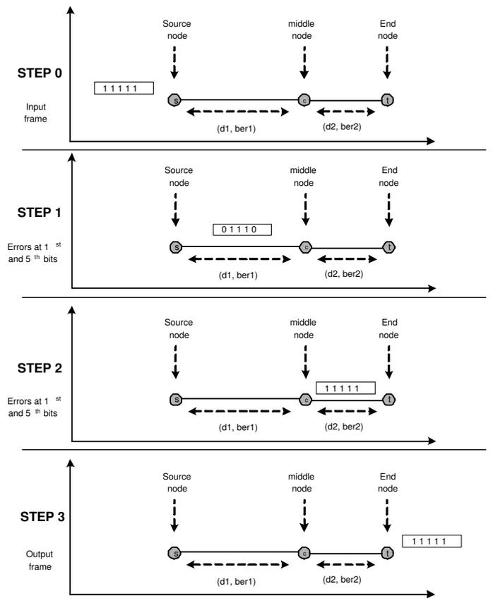
Fig. 1. End-to-end bit error rate case scenario
